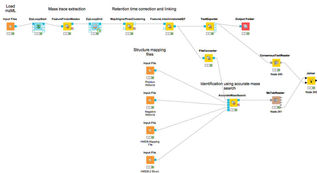
Figure 33: Label-free quantification and identification workflow for metabolites that loads the results into KNIME and joins the tables.
